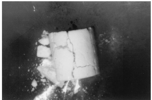
Fig. 11. First cleavage of a larger cylindrical artificial stone (HMT) into several fissures parallel and perpendicular to the wave-propagation direction. The stone dimensions were 10 \times 10 mm. The positive pulse pressure was 31 MPa. The cylinder axis was perpendicular to the wave-propagation direction.
