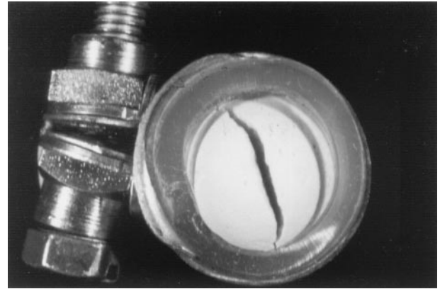
Fig. 7. Cleavage of an artificial stone (HMT 15 mm) by static squeezing. The stone is inserted into a piece of silicon rubber hose and placed in a hose clamp that has been steadily tightened to exert circumferential pressure.
